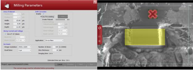
❖ Set up drift correction at last. Choose "use pre-existing" in drift correction and adjust the size and position of red box to cover the Fiducial marker. Click "find" to score Fiducial marker. The score should be as close to 1.00 as possible. If not satisfied with the score click "reset" and adjust Ibeam brightness and contrast to re-score; If satisfied with the score click **NEXT**.
