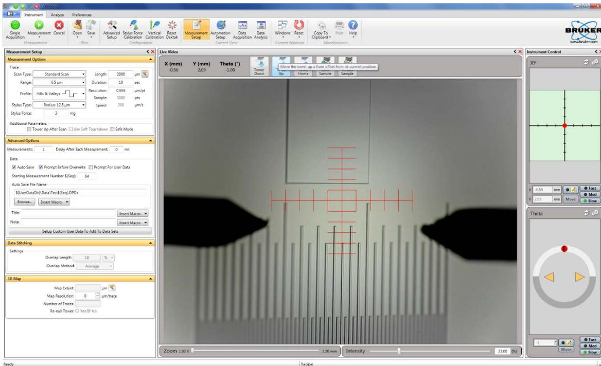
5. In the XY and Theta control panels under Instrument Control, select the speeds at which you want to move and rotate the sample stage.
