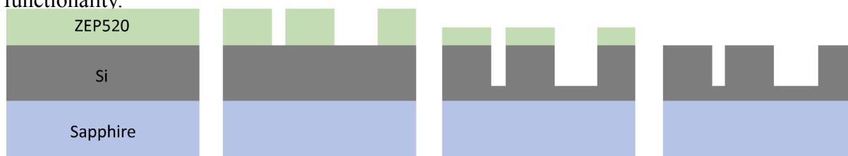
Figure 1. Typical fabrication steps of a metasurface.
