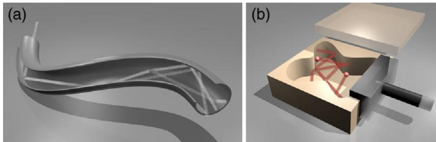
**Figure 1:** Schematics of various multi-mode systems with disorder/chaotic dynamics: (a) A MMF experiencing twists, bendings, and other forms of perturbations along the propagation direction  $z$ ; (b) A multi-mode opto-mechanical cavity) with an incoherently moving wall.
