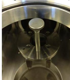
4. Rotate the lid to align it with the chamber. While holding the chamber lid handle, push the lever in toward the post and gently lower the lid into place. (DO NOT DROP THE LID)
